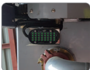
Automatic level status LED display
