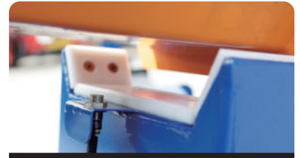
BOOM OUTRIGGER INTERLOCK SENSOR
