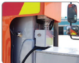
Over-tilt prevention sensor and Safety Check-Valve
