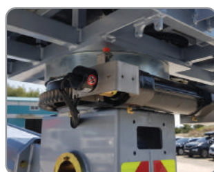
Rotation and Encoder detection
