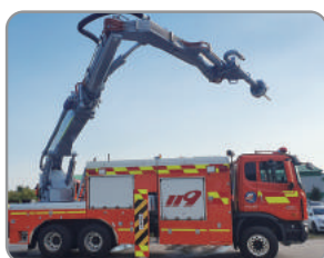
Tri-Axial Articulated Boom movement
