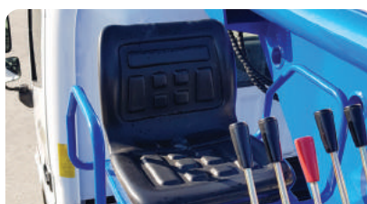
GROUND STATION CONTROL WITH OPERATOR SEAT
