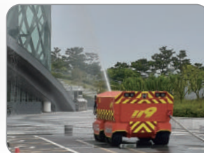
Direct Water Spray or Jet Nozzle auto switching
