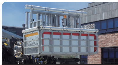
PLATFORM'S LOADING CAPACITY IS 400KG INCLUDING 3 PERSONS
