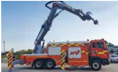
Tri-Axial Articulated Boom movement
