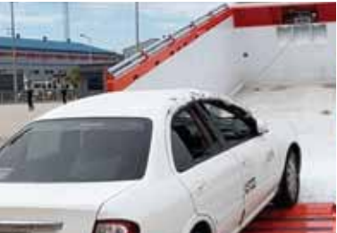
Winch pulling force (Max. 3Ton)
