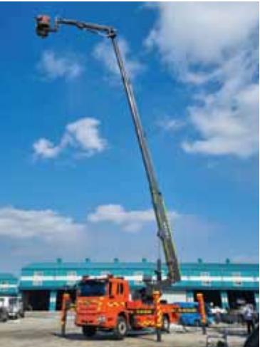
4-Telescopic Booms and 1 Articulating Boom with faster simple operations
