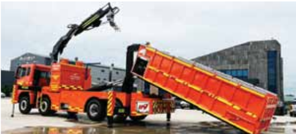
Hookloader for Container movementoption for container
