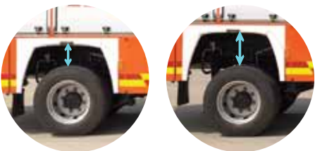
Automatic suspension system to prevent roll-over
