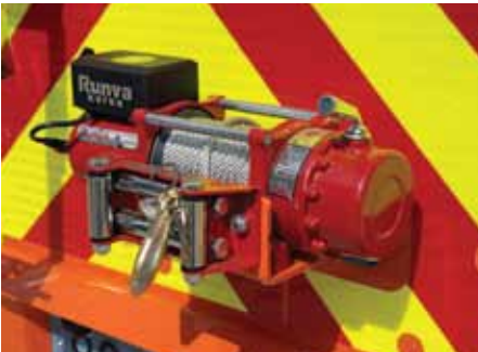
Winch Traction force 1 tons
