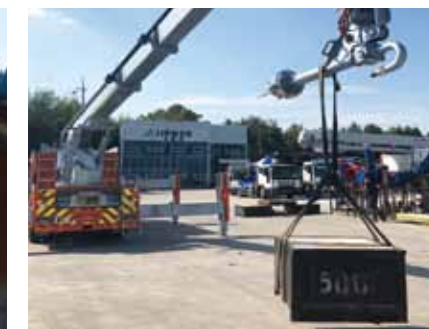
1.5Tons lifting capacity along-with versatile attachment options
