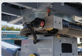
Rotation and Encoder detection
