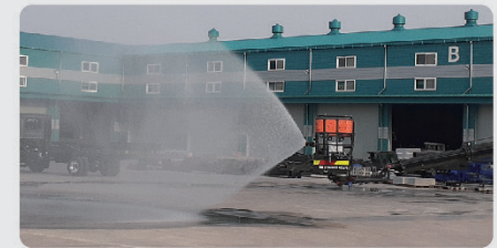
Automatic water turret operations (Spray / Jet)
