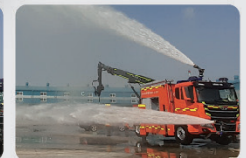
Connective movement by remote control 3 kinds of direct water shooting & spraying
