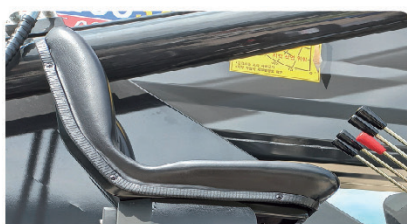
GROUND STATION CONTROL WITH OPERATOR SEAT
