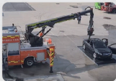
Perforating roof by the piercing destruction tip
