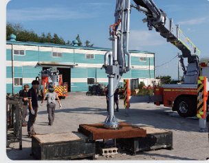
Penetration of Steel plate
