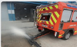
Spraying system of traction device
