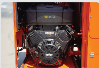
Emergency Auxiliary Engine
